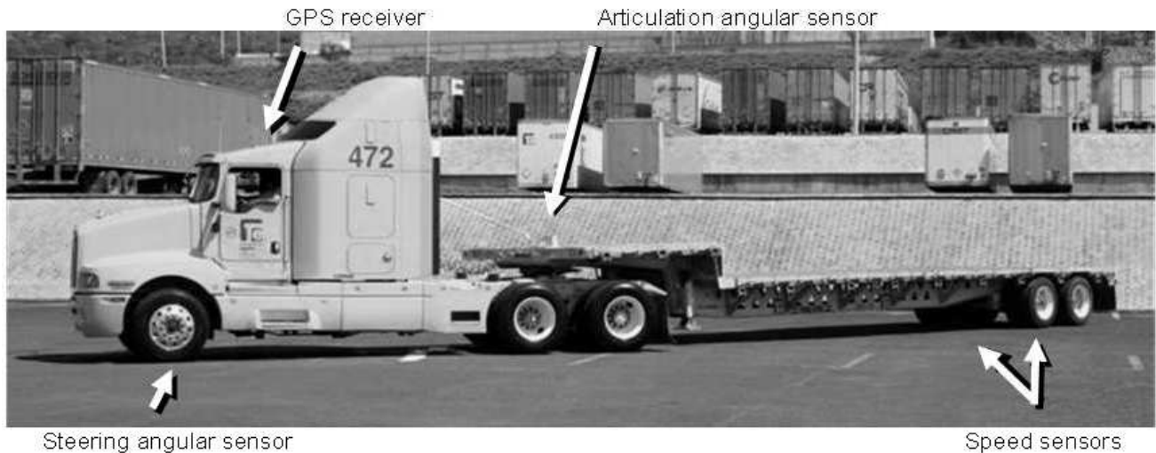
Figure 2 – Instrumented vehicle and sensor location.
