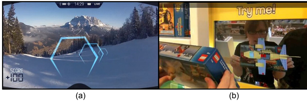
Figure 3.1: Schemes based on the real world and camera relation: (a) World fixed AR, (b) Camera fixed AR
