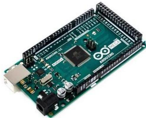
**Figura 3.2** Arduino Mega 2560.
