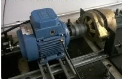
Fig. 6. Induction motor on the test rig.
