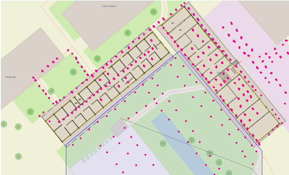
Figure 3.1.: Test area and fingerprint positions ( \cdot ) 8 of one access point. Reference points within the yellow shaded area belong to the Indoor dataset; reference points lying in the blue shaded area form the Outdoor-2 dataset; and all other fingerprints belong to Outdoor-1. © OpenStreetMap contributors
