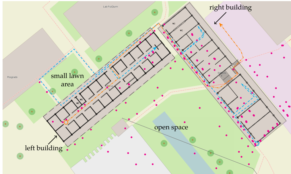
Figure 3.2.: Test area with fingerprint positions ( \bullet ) of one access point and trajectories (Trajectory-1 ---; Trajectory-2 ---). The starting point of each trajectory is marked with a circle and the end point with an arrow. © OpenStreetMap contributors © IEEE 2015
