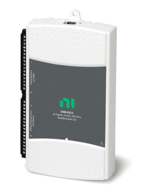
Figura 8. NI-USB 6211 (Instruments, 2019).
