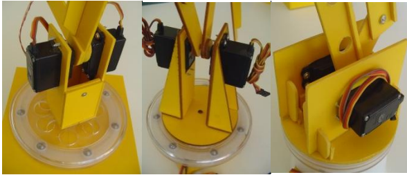
Figure 6. Examples of motor base rotating bearing table assemblies.
