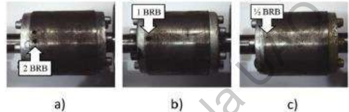
Fig. 2. Arrangement of the different faults produced in the experimental test bench. (a) 2 Broken rotor bars. (b) 1 Broken rotor bar. (c) 1/2 Broken rotor bar.
