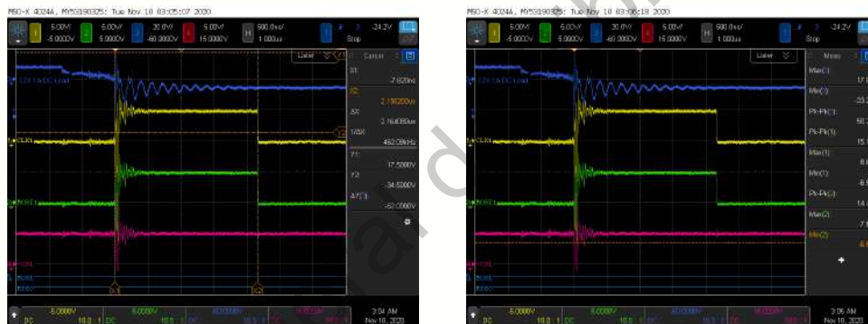
Figure 5.12: Voltage spikes on the data lines
