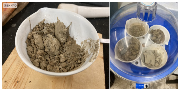
Figure 6: Shredding and moisture extraction.
