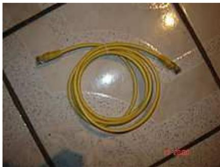
**Figura 2.33** Cable de Ethernet.
