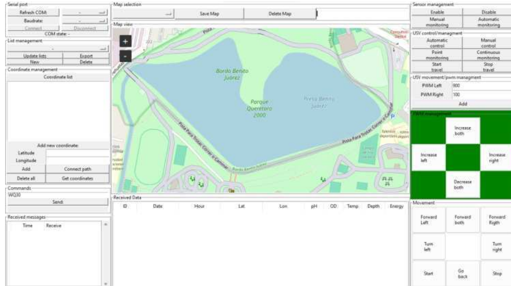
Figure 5.13: Graphical user interface for USV controlling.
