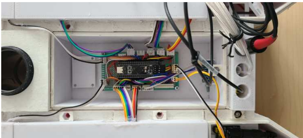
Figure 5.8: Superior view of the main circuit hull.
