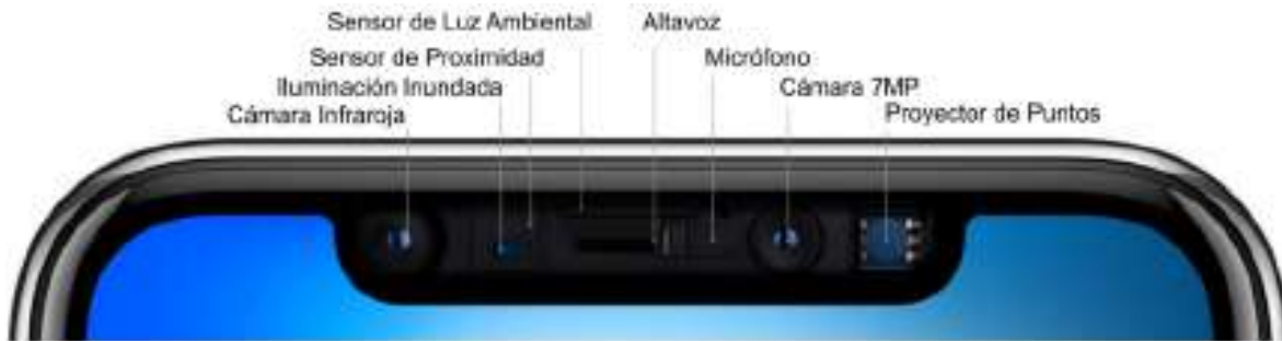
Figura 1.15: Sensor iPhone X TrueDepth (LeCompte et al., 2019).
