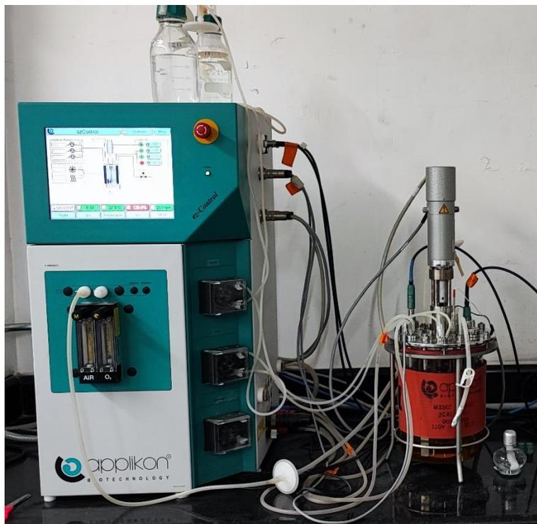
**Figura 25.** Biorreactor instrumentado Applikon ez-control, modelo Z31011001.
