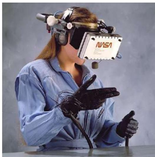
Fig. 30: Virtual Interface Environment Workstation “VIEW”, NASA / S.S. Fisher, W. Sisler. (1988)
