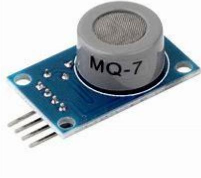
*Figura 3: sensor MQ-7 (Geek factory, s.f.)*
