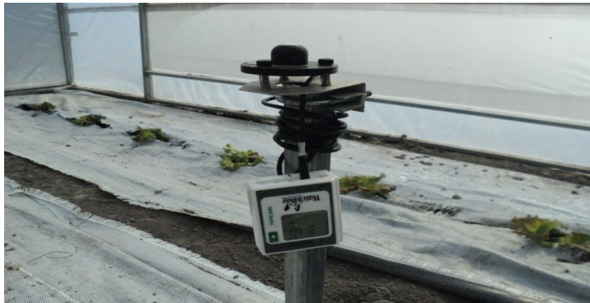
Figura 3.6 Data logger Watch Dog.
