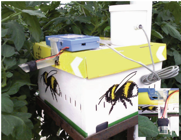
Fig. 1. Bee activity recorder in place on a bumble bee hive. (Online figure in color.)
