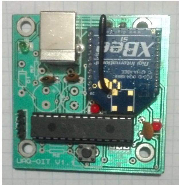
Figura IV.19 Tarjeta USB-Serial a XBee.
