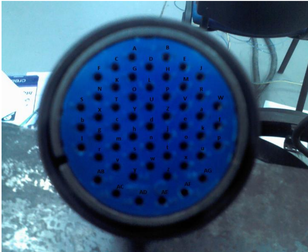
Figura 2.12. Conector hembra del cable de control general CNR01A, CNR01, CNR02, CNR04 Y CNR010.
