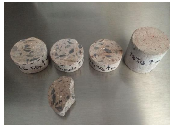
Fig. 8. Stained concrete with textile painting carmine red color to a concentration 100 ppm (after 4 hours of exposure)
