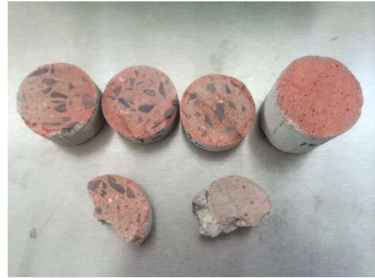
Fig. 7. Stained concrete with textile painting carmine red to a concentration 100 ppm (before exposure)
