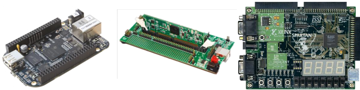
Figura 2.15 Beagle Bone Black, DSP C200 y FPGA Spartan6
