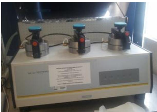
**Figura 6.** Equipo VAC-V2 Gas Permeability Tested (Labthink Instruments Co., Ltd, China)
