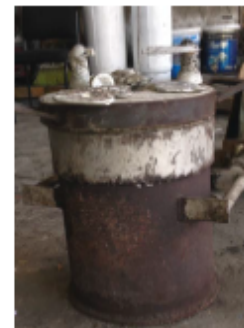
Figure 1. Furnace used. Supplied with a gas tank and a silicon carbide crucible.
