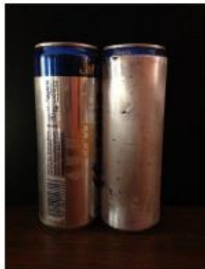
Figure 2. Cans before and after lacquer removal.
