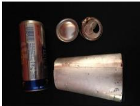
Figure 3. Aluminum can completely treated. Lacquer, top and base removed.
