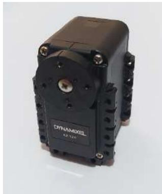
**Figura 3.6** Servomotor Dynamixel AX-12A.
