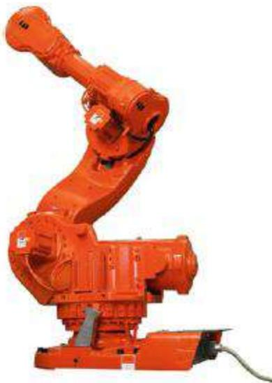
**Figura 1.1.** Robot Manipulador Serial (*Fundamentals of Robotic Mechanical Systems*, 2014).
