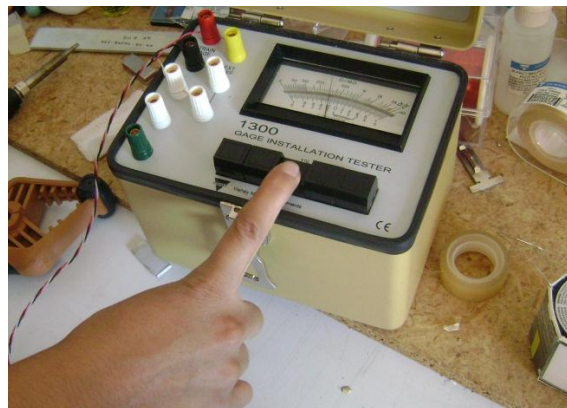
Figura 3.10. Gauge instalation Tester 1300
