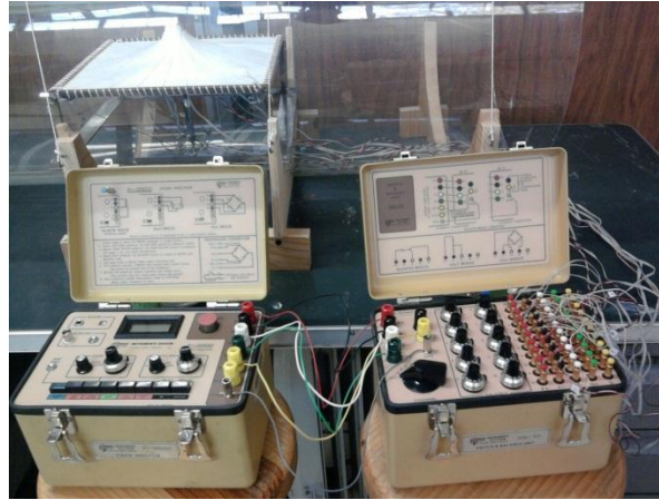
Figura 3.11. Strain Indicator P-3500 y Switch and Balance Unit
