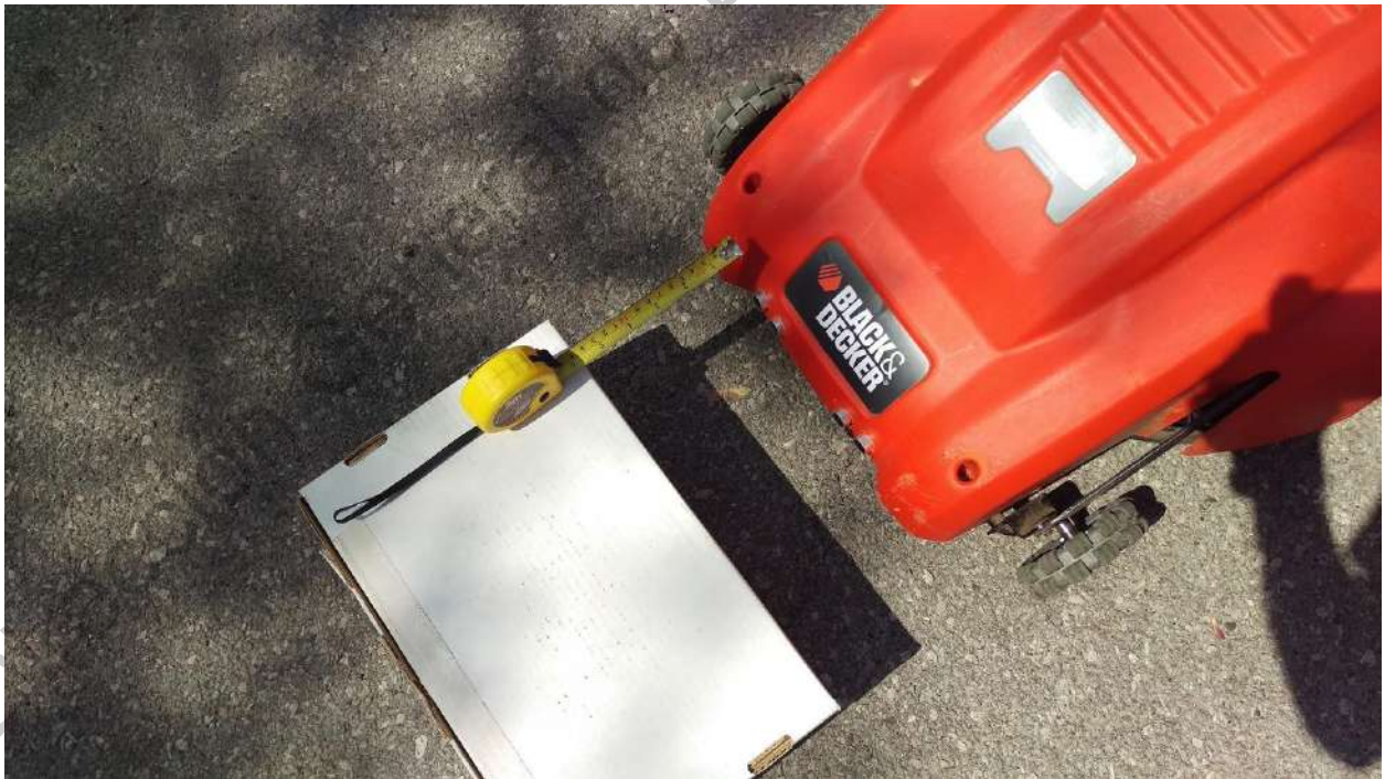
Figure 54. The vehicle stopped in concrete when an obstacle was detected (example of obstacle 2).
