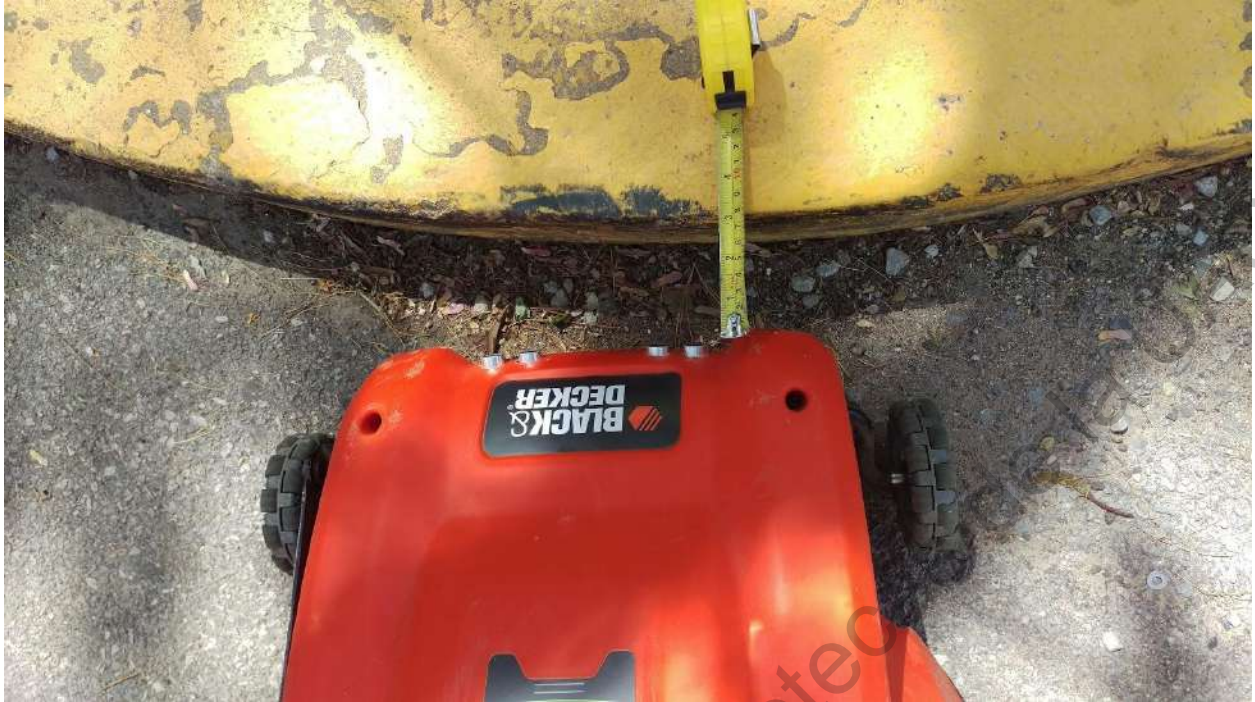
Figure 53. The vehicle stopped in concrete when an obstacle was detected (example of obstacle 1).
