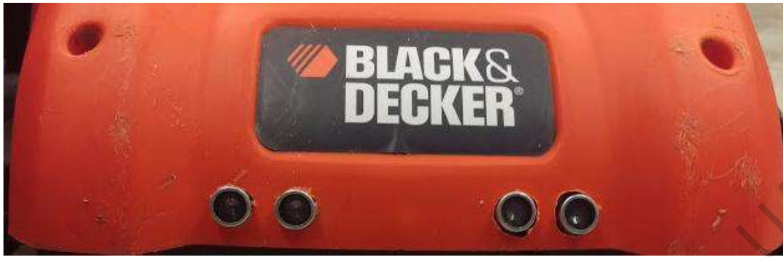
Figure 37. Free of obstruction ultrasonic sensors.
