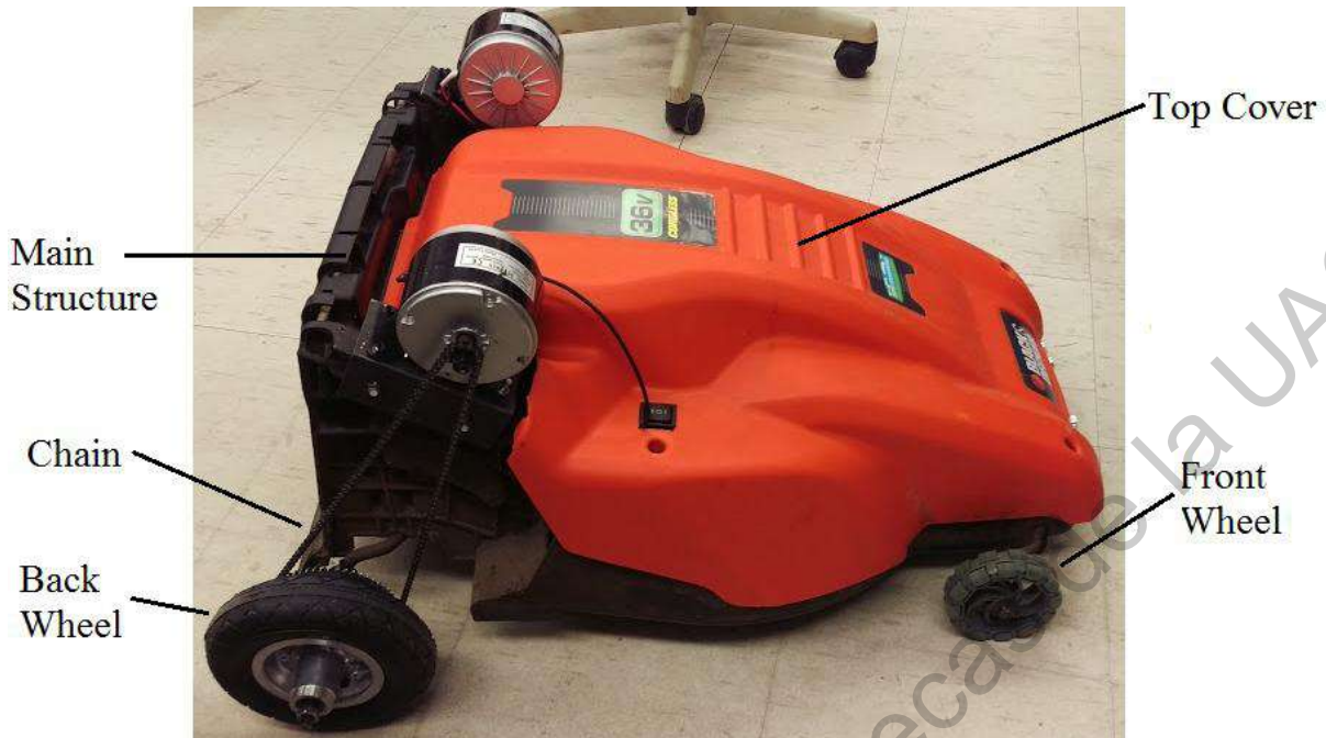
Figure 36. Lawn mower (side view) with main components.
