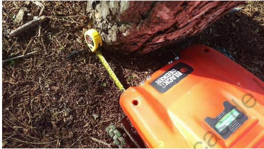
Figure 58. The vehicle stopped when an obstacle was detected (example of obstacle 2).
