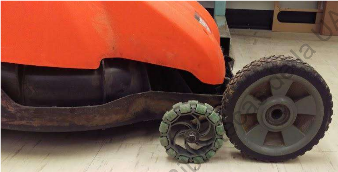
Figure 25. Comparison between omnidirectional mounted and original wheel.
