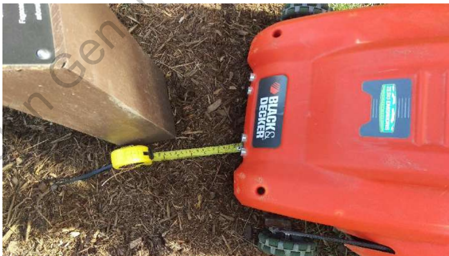
Figure 57. The vehicle stopped when an obstacle was detected (example of obstacle 1).
