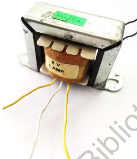
Figure 3.7 6 V output transformer.
