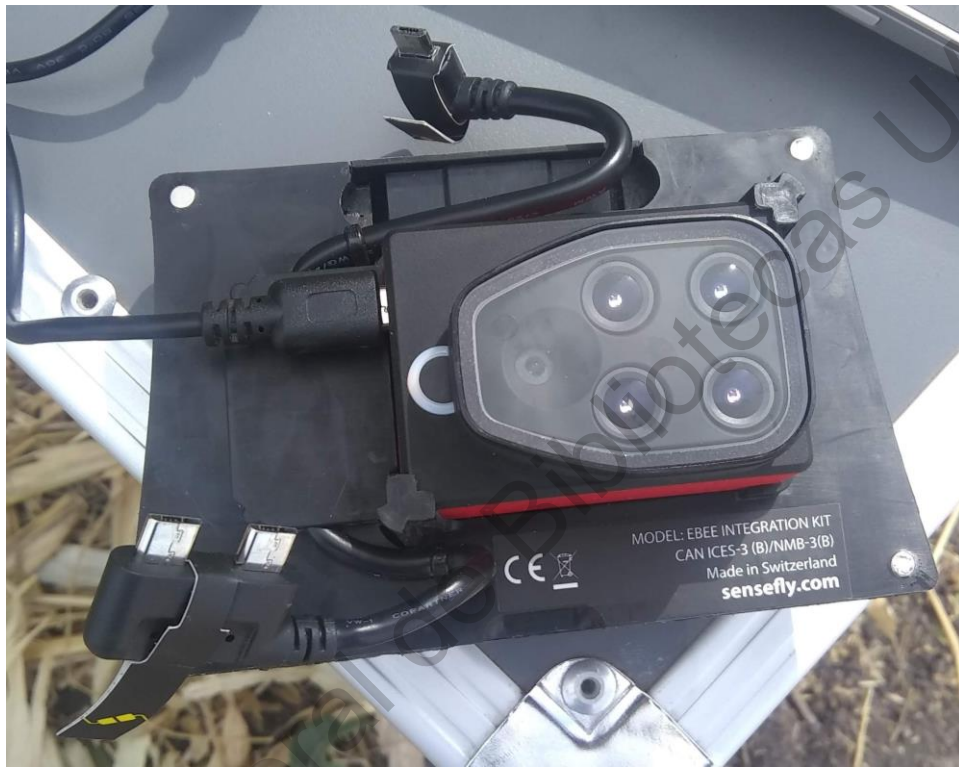
Figura 8. Sensor multispectral Parrot Sequoia
