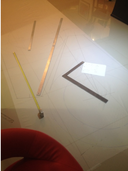
6-45. Tracing and cutting tools for real scale hoops
