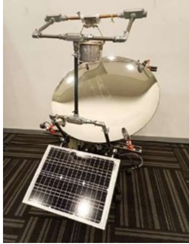
Figure 3.5: One-degree-of-freedom solar collector used in the experimental plant [2].
