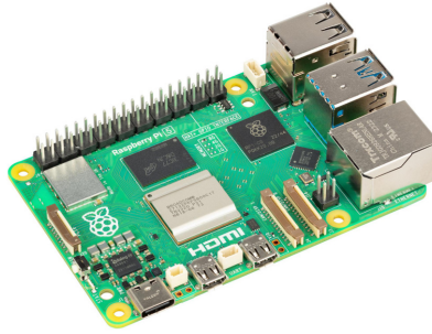
Figura 5.6: Tarjeta Raspberry Pi 5 [27].
