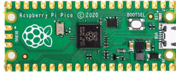
Figura 5.5: Microcontrolador Raspberry Pi Pico [26].
