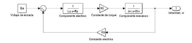
Note. Block Diagram was developed by the author to represent the DC motor model. This is based on different Control Engineering literature.
