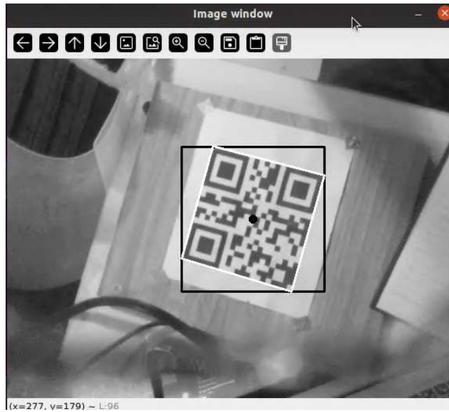
Figure 3.8: QR marker detected with YOLOv8 QRDet. The QR is segmented and surrounded by the bounding box.
