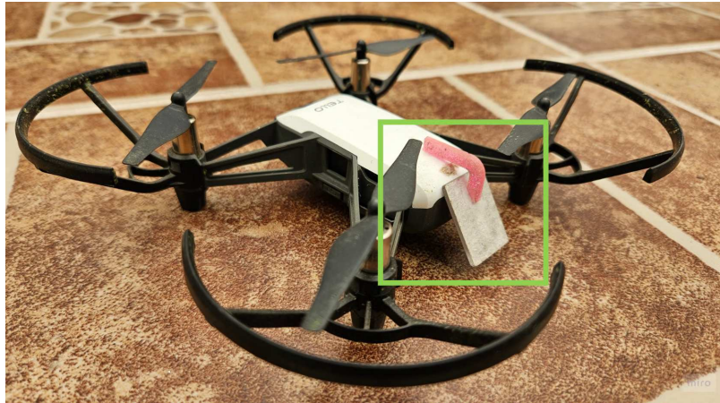
Figure 3.2: Tello drone equipped with a 2x2.5 cm mirror angled at 45° to direct the camera's view downward.
