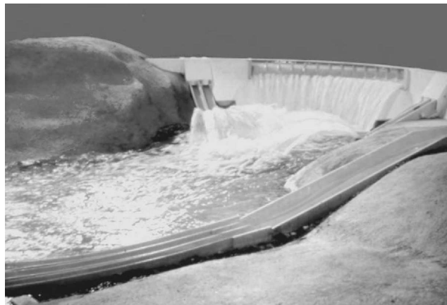
Cha 3 fig 1 Laboratory model of a dam spillway
