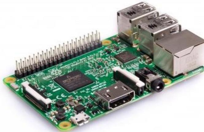
**Figura 3-4. Raspberry Pi 3 modelo B. Fuente: Raspberry Pi (McGrath, 2016).**
