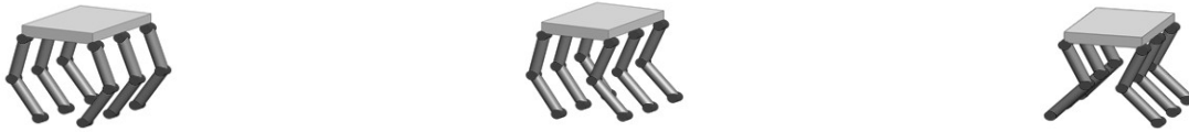
Fig. 2. (a) Knees outwards; (b) Knees with the same orientation; (c) Knees inwards.
