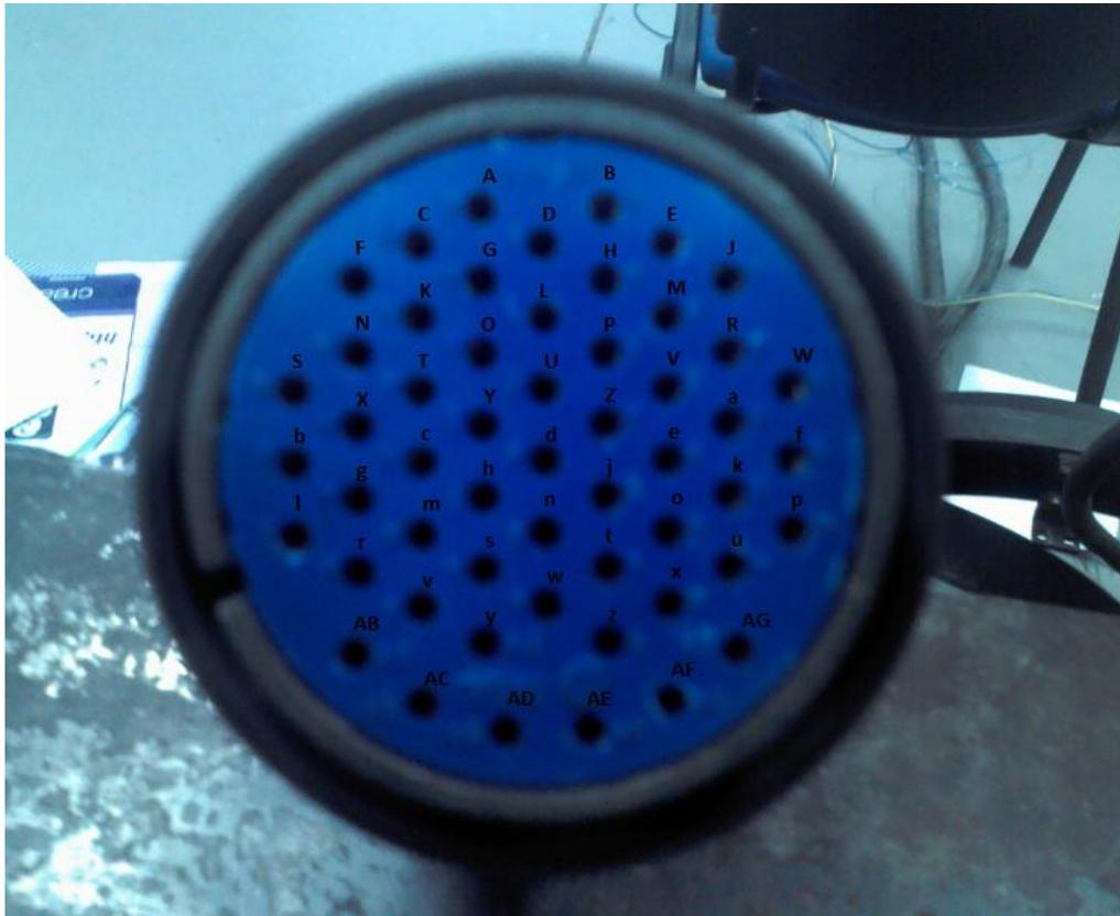
**Figura 2.12.** Conector hembra del cable de control general CNRO1A, CNRO1, CNRO2, CNR04 Y CNR010.
