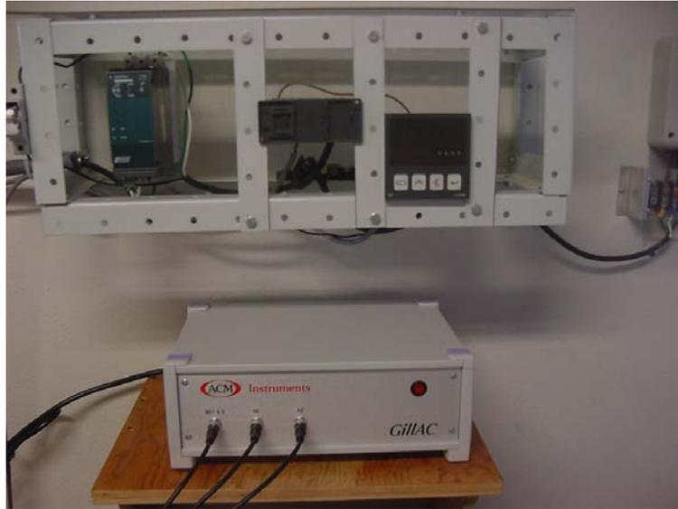
Figura 3.5 Potenciostato Gill AC
