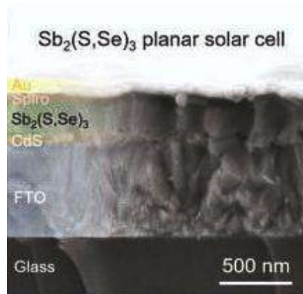
Fig. 4. Experimental high performance Sb_2(S,Se)_3 solar cell device structure.
