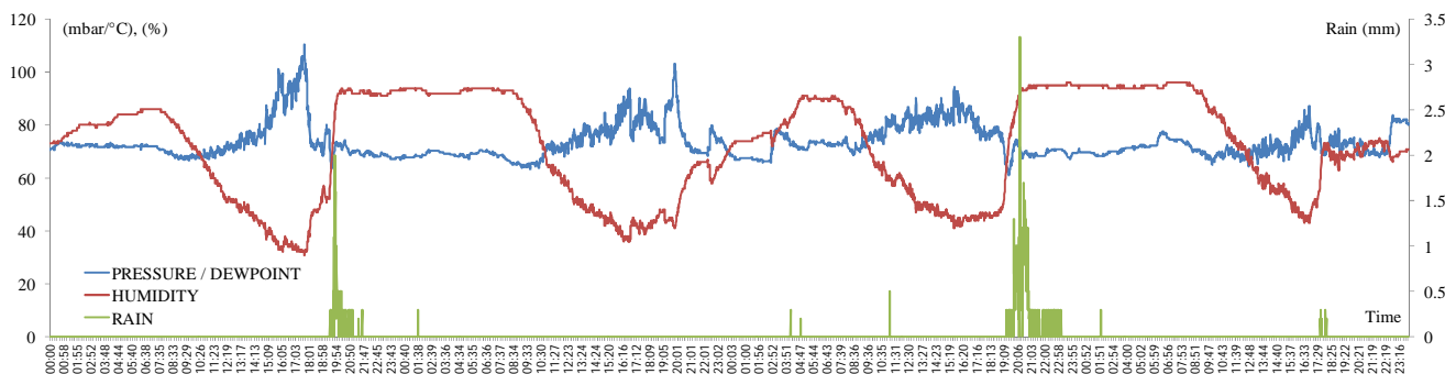
Figure 4. Results of the application of the CRHUDA model to the AWS-UAQ Cerro Campanas data of 16 August 2014 (maximum rainfall 55.2 mm in 1-h; maximum intensity 63.8 mm/h; 53-year return period).
