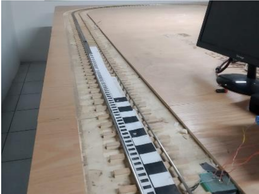
Figure 4.14 The area where braking experiments are conducted; approximately 2.5 meters long, from the curve to the center of the test bench.
