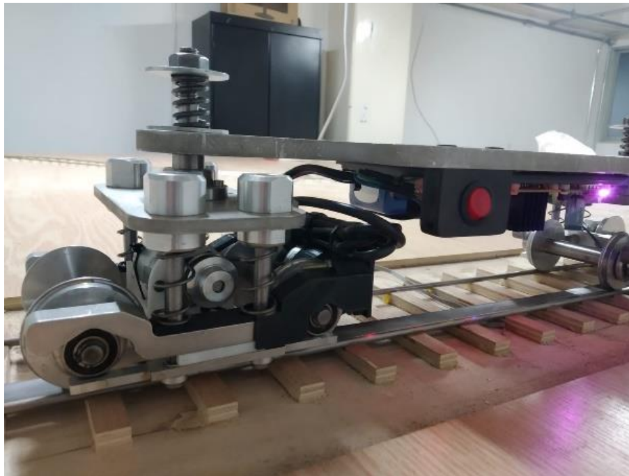
Figure 4.13 Position of the test vehicle before the start of the experiment. To prevent the optical sensor from activating before the braking zone, a black tape was placed over the track.
