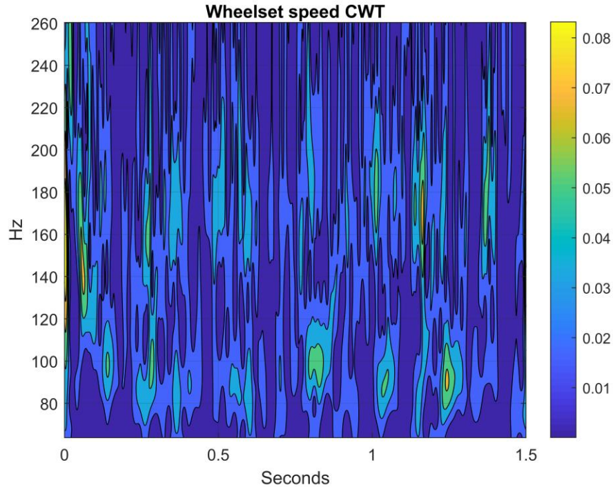
Figure 5.22 Results of the wheelset's CWT while braking on greased rails. The yellow areas represent frequencies with the greatest amplitude. Multiple short-duration frequencies stand out. In contrast to the no-brake scenario, a more regular pattern is observed here: one with low frequencies around 80 Hz and one with high frequencies around 180 Hz.
