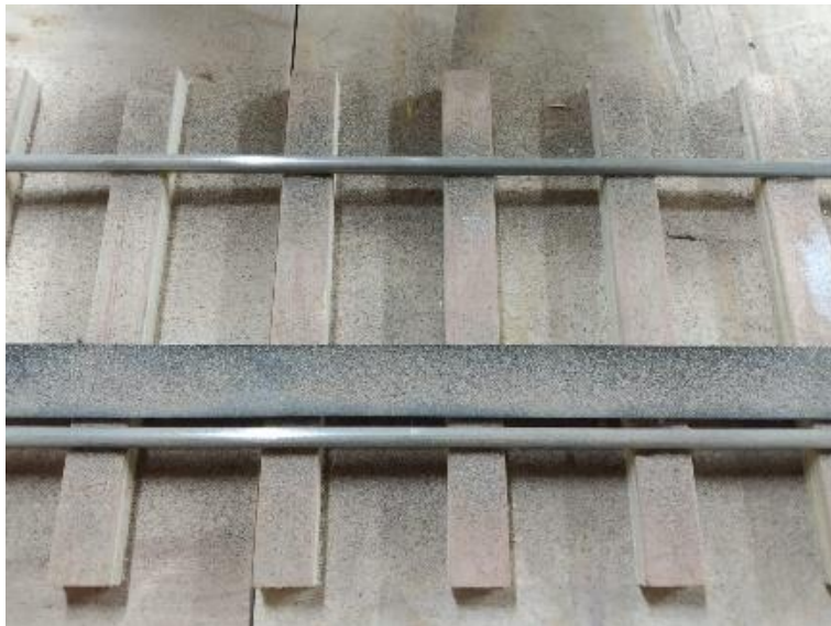
Figure 4.11 Sand-scattered rails. The sand was spread across the entire braking zone.
