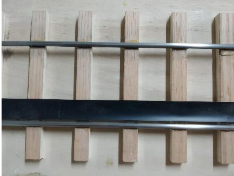
Figure 4.10 Clean rails. Wheels and rails were cleaned to remove any traces of contamination.
