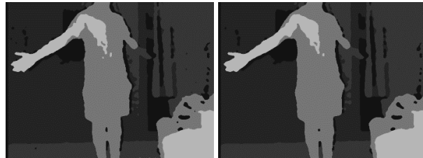
a) Median filter kernel size 9x9 b) Median filter kernel size 11x11
