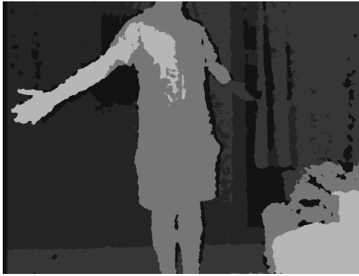
Fig. 10. Kinect depth image with noise and holes
